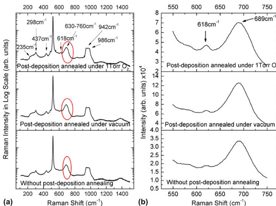
FIG. 5. The Raman spectra of thin films grown without postdeposition annealing, postdeposition annealing under vacuum, and postdeposition annealing under 1 Torr O<sub>2</sub> atmosphere (a) in the full range and (b) in the interval of 550–750 cm<sup>-1</sup>.
