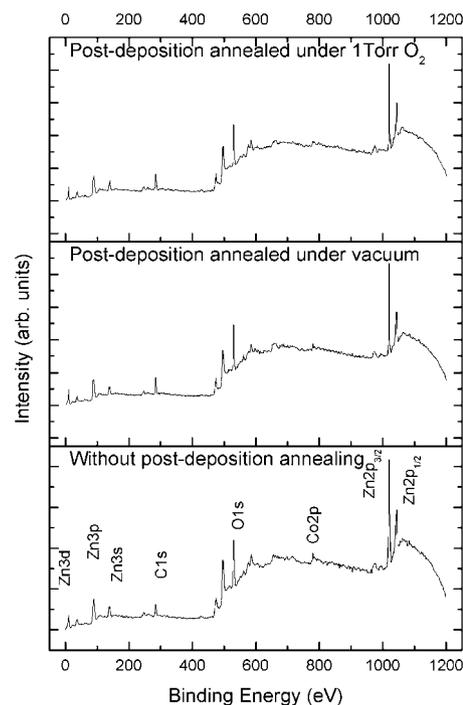
FIG. 3. XPS spectra of the films grown from  $\text{Zn}_{0.90}\text{Co}_{0.10}\text{O}$  target without the postdeposition annealing, postdeposition annealing under vacuum atmosphere, and postdeposition annealing under 1 Torr  $\text{O}_2$  atmosphere.
