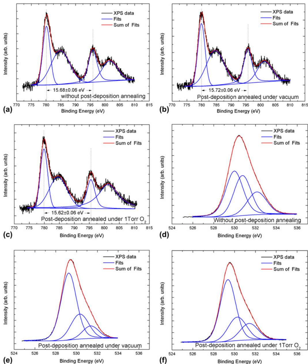
FIG. 4. XPS spectra of (a)–(c) the Co 2p (in binding energy range of 770 and 815 eV) and (d)–(f) O 1s (in binding energy range of 524 and 537 eV) energy levels for the films deposited by Zn<sub>0.90</sub>Co<sub>0.10</sub>O target without postdeposition annealing, postdeposition annealing under vacuum, and postdeposition annealing under 1 Torr O<sub>2</sub> atmosphere, respectively.
