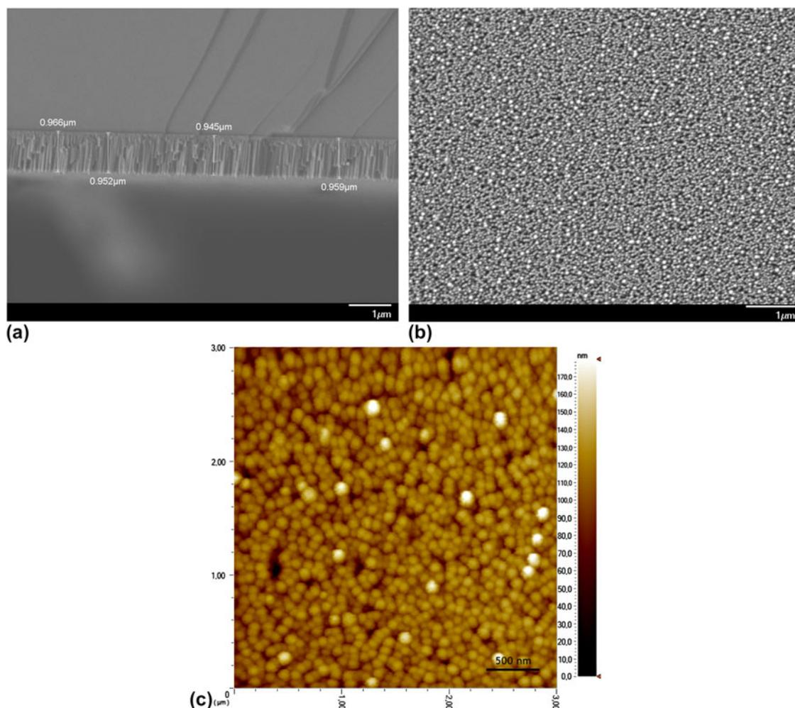
FIG. 2. The SEM micrographs of (a) cross-sectional thickness and (b) surface morphology and (c) the AFM image of Zn<sub>0.9</sub>Co<sub>0.1</sub>O films without postdeposition annealing.
