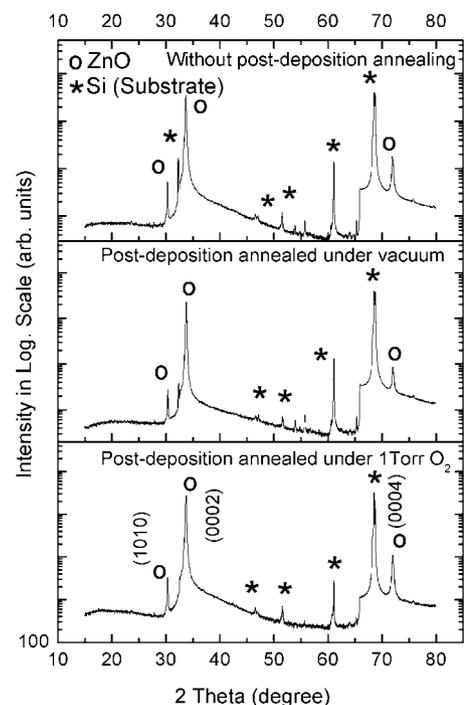
FIG. 1. XRD patterns of the films grown from Zn<sub>0.90</sub>Co<sub>0.10</sub>O target without postdeposition annealing, postdeposition annealing under vacuum atmosphere, and postdeposition annealing under 1 Torr O<sub>2</sub> atmosphere.
