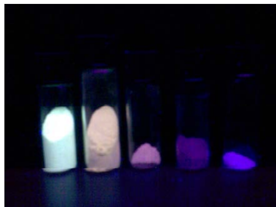
Fig. (1). Physical appearance of prepared ZnO quantum dots under UV lamp (345 nm).
