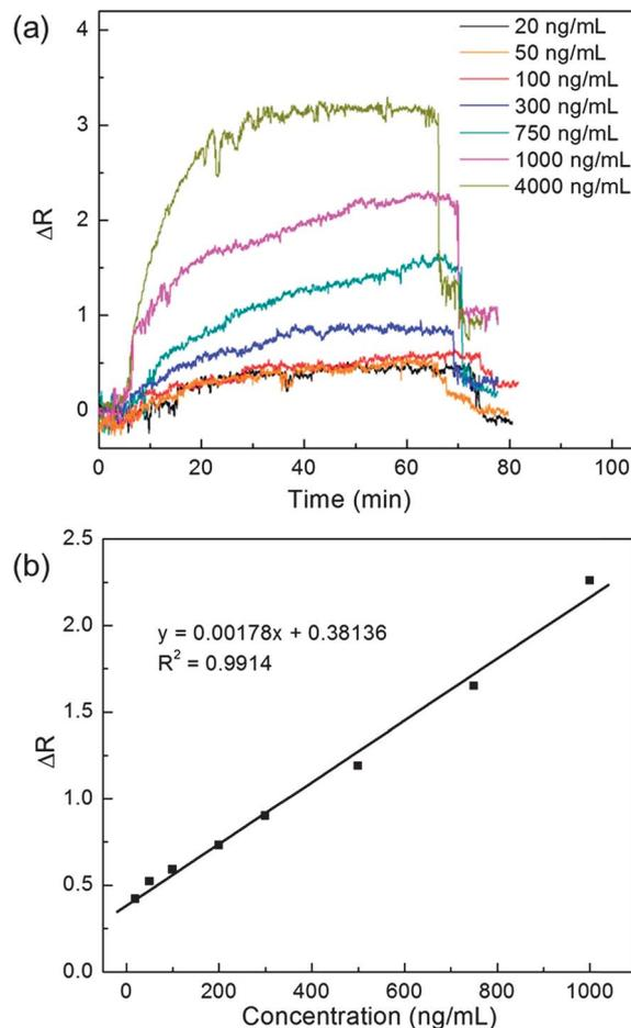
**Fig. 2** (a) Real-time response of a SPR biosensor against several PCT solutions in phosphate buffer at different concentrations. (b) Concentration dependency of a PCT imprinted SPR biosensor showing the high linearity of the sensor response in the studied concentration range.
