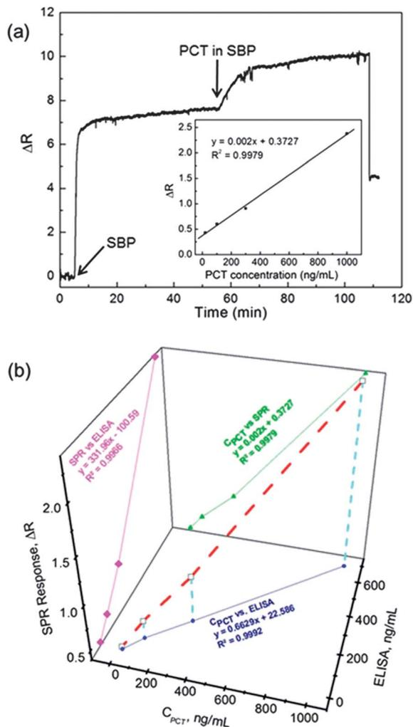
**Fig. 4** (a) Typical real-time response of a SPR biosensor against PCT solutions in simulated blood plasma (SBP) at  $1000 \text{ ng mL}^{-1}$ . The inset shows the concentration dependency of a PCT imprinted SPR biosensor showing the high linearity of the sensor response in the studied concentration range. (b) Comparison of PCT detection results of the SPR biosensor with the results of the ELISA test.
