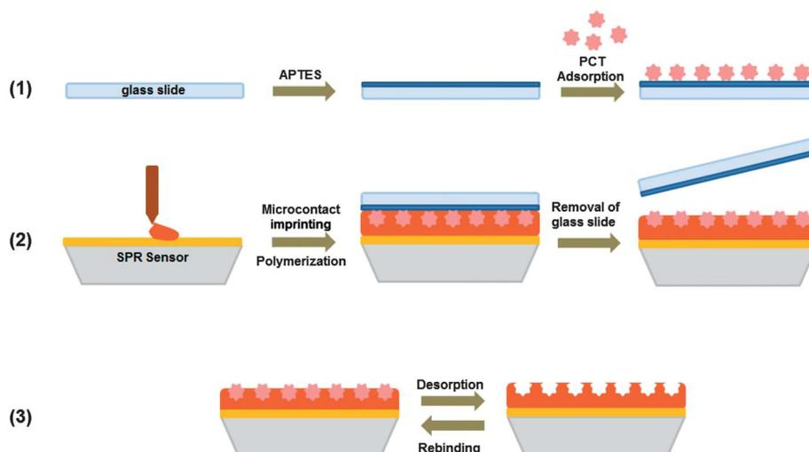
**Scheme 1** Schematic representation of the microcontact PCT imprinted SPR biosensor fabrication.
