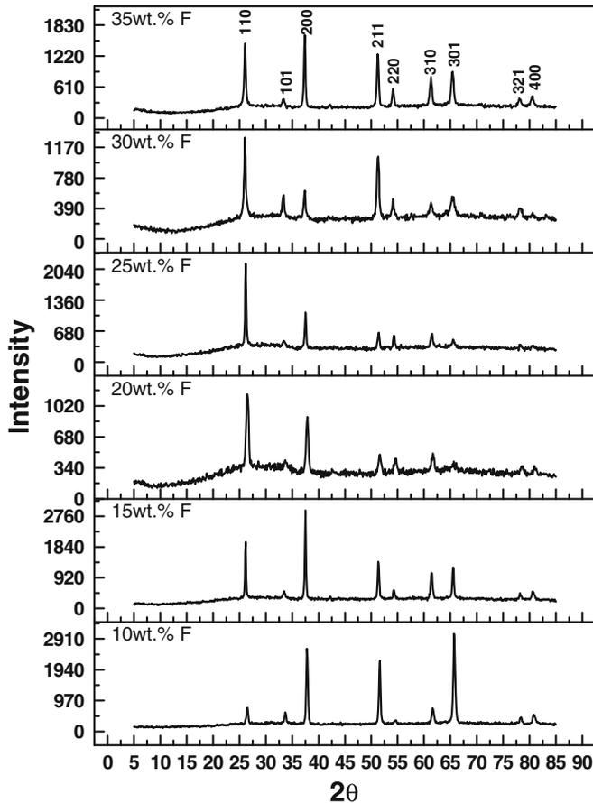
**Figure 2.** XRD spectra of the FTO films deposited on glass at different concentrations.
