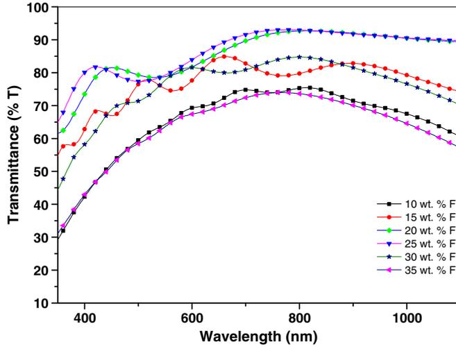
Figure 5. Optical transmission spectra of FTO thin films as a function of F-doping concentration.
