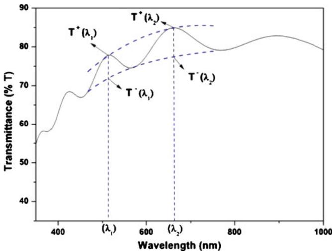
Figure 6. Transmission curve of interference envelope functions  $T^+(\lambda)$  and  $T^-(\lambda)$ .
