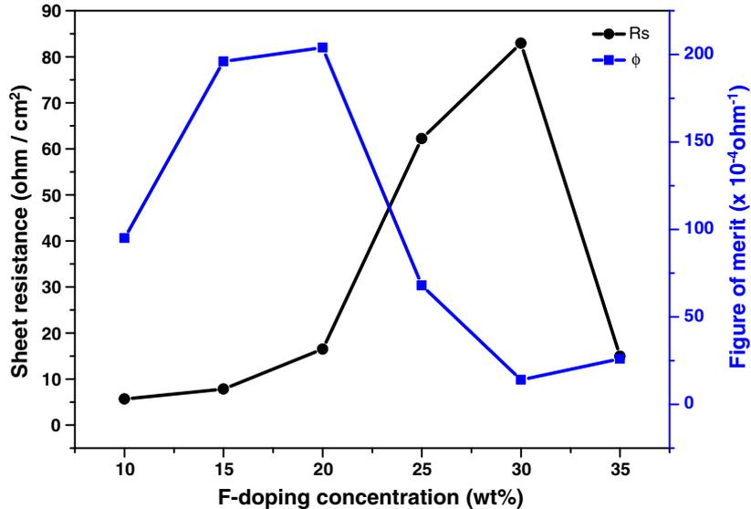
**Figure 8.** Plot of sheet resistance and figure-of-merit as a function of F-doping concentration.
