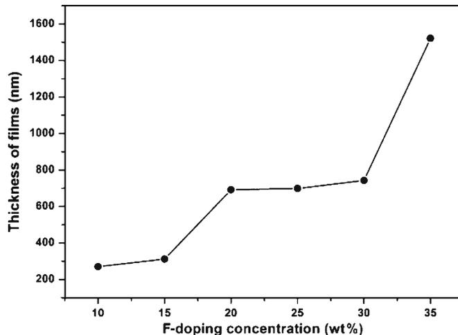
Figure 7. Variation of the film thickness of FTO thin films as a function of F-doping concentration.
