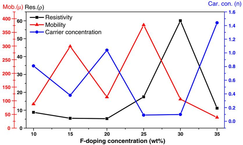
**Figure 3.** Resistivity, mobility and carrier concentration of FTO films as a function of F-doping concentration.
