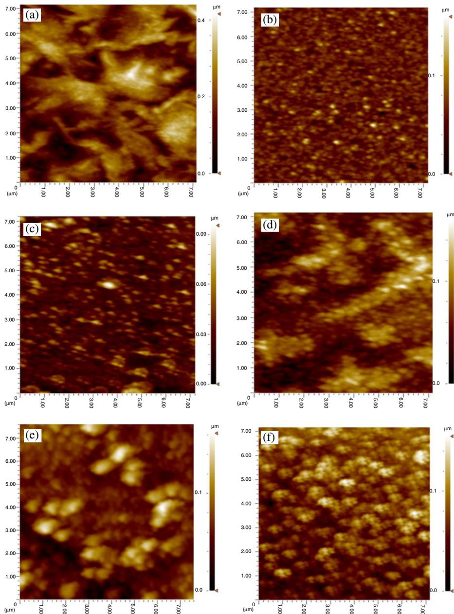
**Figure 1.** The AFM surface 2D images of FTO films as a function of F-doping concentrations: (a) 10 wt.%, (b) 15 wt.%, (c) 20 wt.%, (d) 25 wt.%, (e) 30 wt.%, (f) 35 wt.%.
