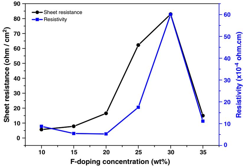
**Figure 4.** Variation of sheet resistance and resistivity of SnO<sub>2</sub>:F films with different fluorine concentrations.
