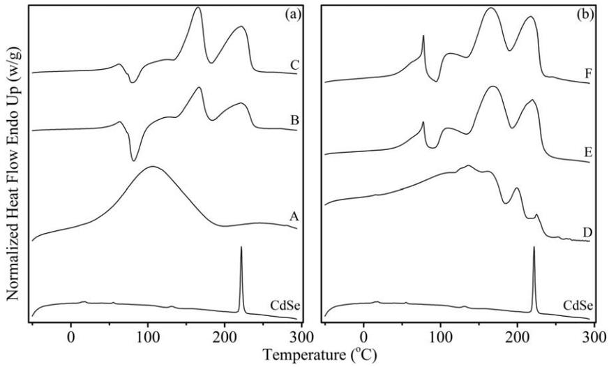
FIG. 7. (a) DSC thermograms of (a) 3:1 PIN and (b) 3:2 PIN and their nanocomposites.
