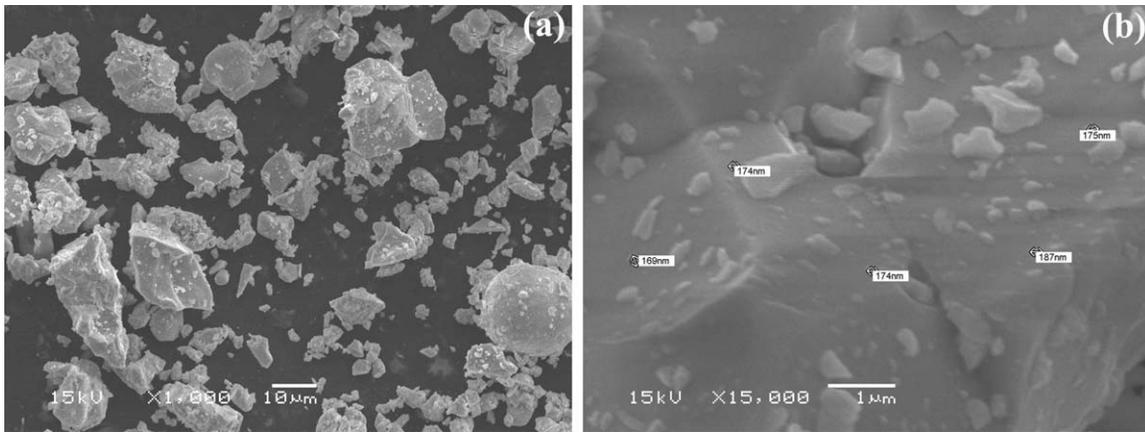
FIG. 4. SEM micrographs of CdSe nanoparticles at magnifications of (a) 1k and (b) 15k.
