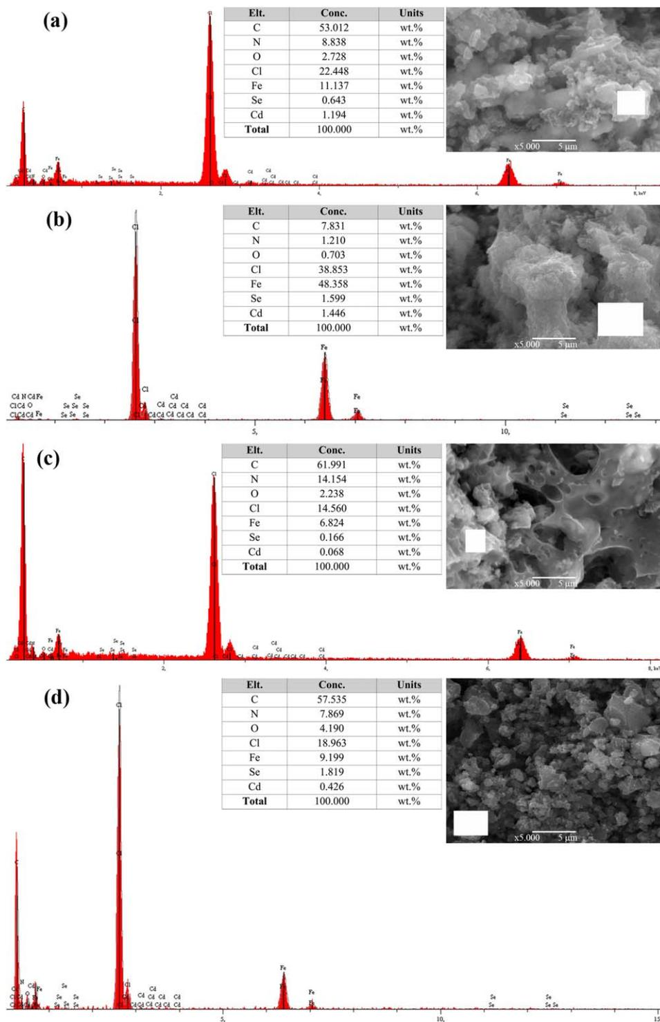
FIG. 2. SEM-EDX analyses of nanocomposites. (a) B, (b) C, (c) E, and (d) F. [Color figure can be viewed in the online issue, which is available at [wileyonlinelibrary.com](http://wileyonlinelibrary.com).]
