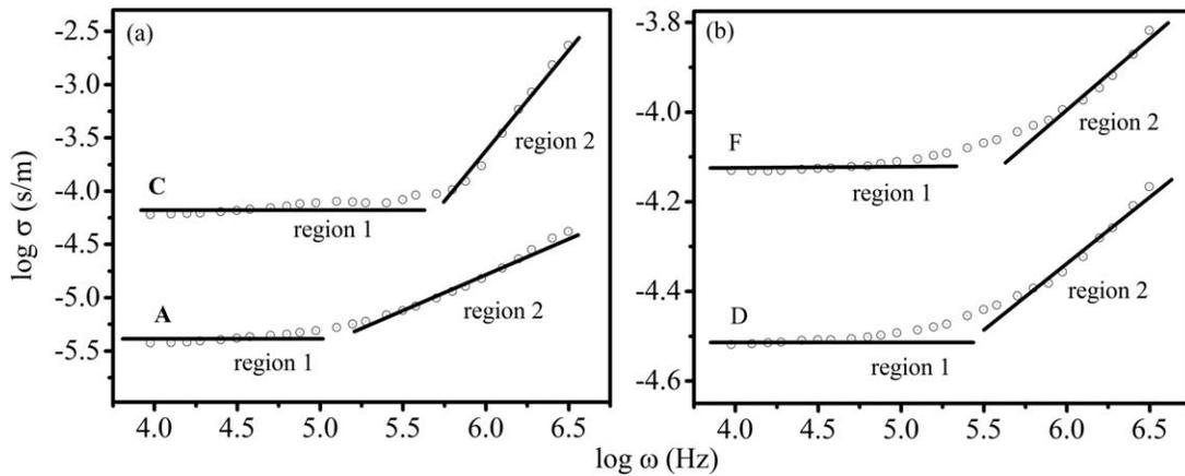
FIG. 9. Frequency dependence of ac conductivity of (a) samples A and C, (b) samples D and F at 300 K.
