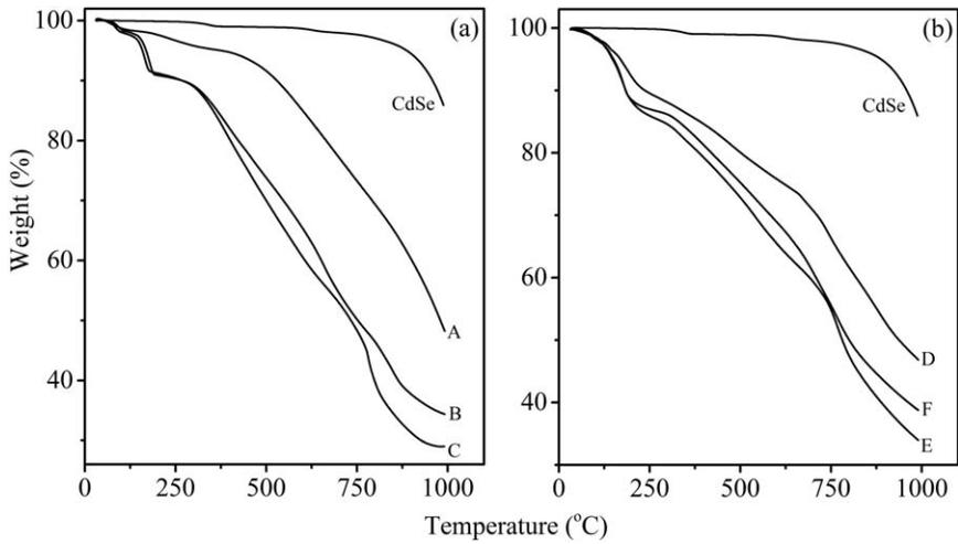
FIG. 8. TG curves of (a) 3:1 PIN and (b) 3:2 PIN and their nanocomposites.
