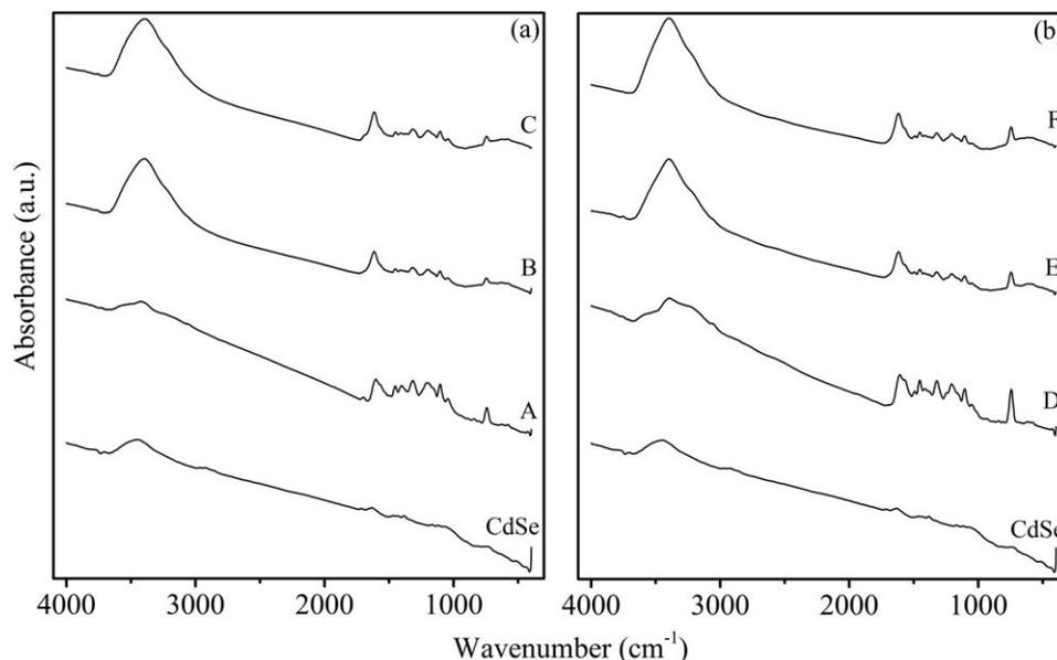
FIG. 1. FT-IR spectra of (a) 3:1 PIN and (b) 3:2 PIN and their nanocomposites.
