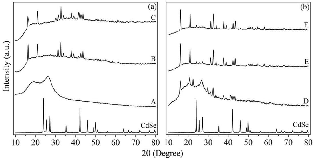
FIG. 3. X-ray diffraction patterns of (a) 3:1 PIN and (b) 3:2 PIN and their nanocomposites.
