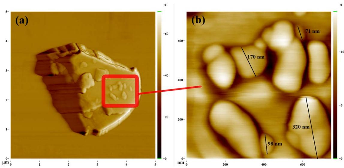
FIG. 5. AFM phase image of CdSe nanoparticles. [Color figure can be viewed in the online issue, which is available at [wileyonlinelibrary.com](http://wileyonlinelibrary.com).]
