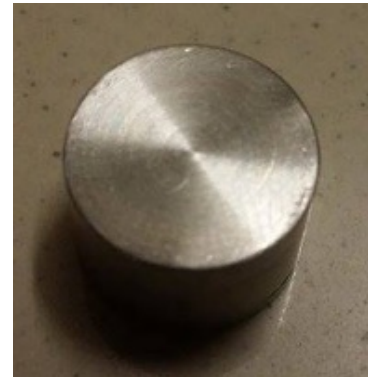
Fig. 2. Cut sample of Inconel 718 obtained by abrasive cutting with water as coolant in Labotom-5.
