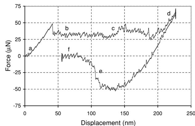
**Figure 7.** The load–displacement curve obtained from a series of TEM images. While unloading there is an attractive force on the indenter corresponding to the material being pulled out of the sample—stages e and f.
