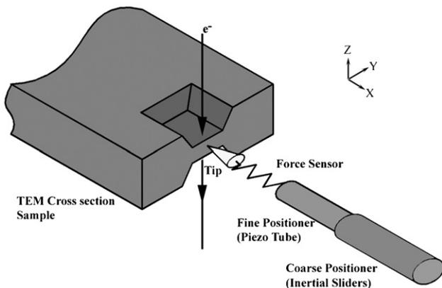
**Figure 1.** Schematic of the TEM nanoindenter. The indentation axis ( $x$ ) is perpendicular to the optic axis ( $z$ ) enabling the deformation to be observed in the transmission electron microscope.
