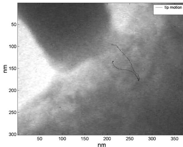
**Figure 6.** TEM image showing the copper sample being indented by a tungsten tip. The curve at the centre of the image shows the trajectory of the tip during the loading–hold–unloading cycle.
