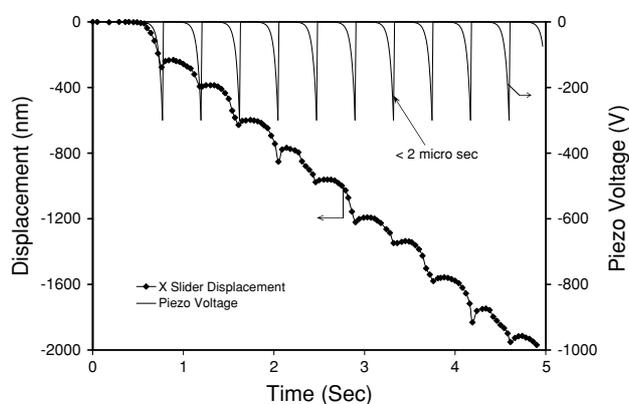
**Figure 4.** Performance of the coarse X-slider. The continuous line shows the waveform applied to the piezo. The resulting slider displacement (filled diamonds) is measured with the help of a heterodyne interferometer.
