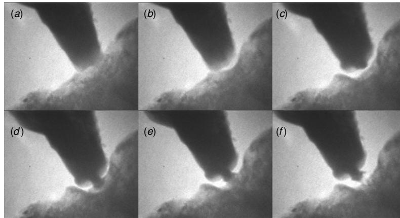
**Figure 8.** TEM images showing different stages during indentation of a fractured copper surface. The stages, (a)–(f), represent distinct events taking place in the load–displacement curve as marked in figure 7. Each image is of size  $1500 \times 1000 \text{ nm}^2$
