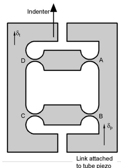
**Figure 5.** Schematic of the nanoindenter force sensor based on four flexible hinges marked as A–D. These hinges form a four bar mechanism that ensures the indenter moves in a straight line with respect to the piezo.
