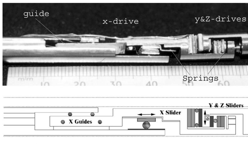
**Figure 3.** Image and schematic of the three-axis coarse positioner. The springs help to adjust the frictional force at the ball–plate interfaces.
