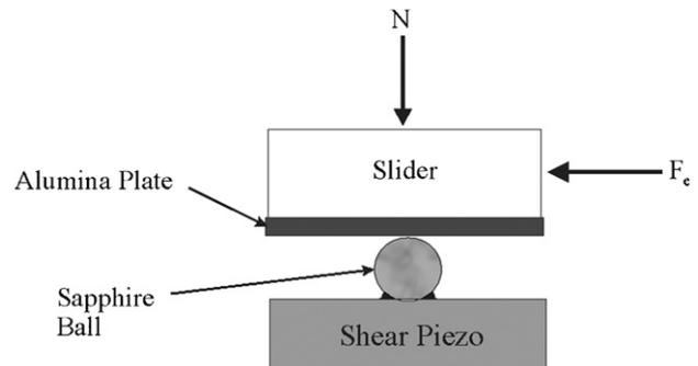
**Figure 2.** Schematic of the inertial slider.  $N$  is the force normal to the sapphire–alumina contact plane and  $F_c$  is the frictional force in the contact plane. The ball slips against the slider if the inertial and external forces are greater than the frictional force.
