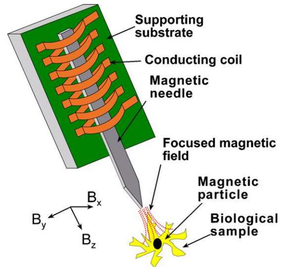
Fig. 1. Schematic of the micro electromagentic probe to be developed. The probe consists of a supporting substrate, a solenoid conducting coil and a protruding (Permalloy) magnetic core with a sharp tip that allows interaction with biological samples.
