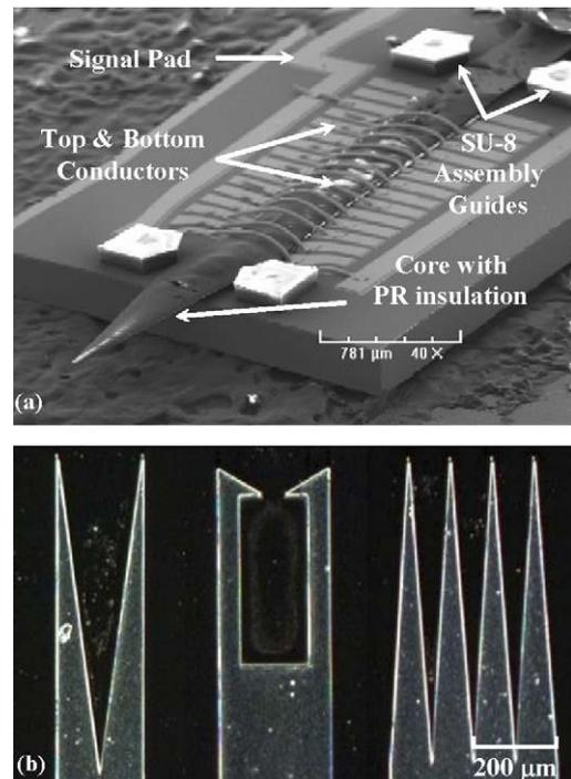
Fig. 4. (a) Scanning electron micrograph of a fabricated micro electromagnetic probe; (b) optical microscopy pictures of Permalloy magnetic cores with different tip profiles.
