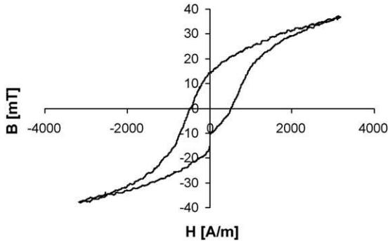
Fig. 8. The  $B$ – $H$  curve of the Permalloy magnetic core characterized by the scanning Hall probe microscope located about  $20\ \mu\text{m}$  from the tip of the core.
