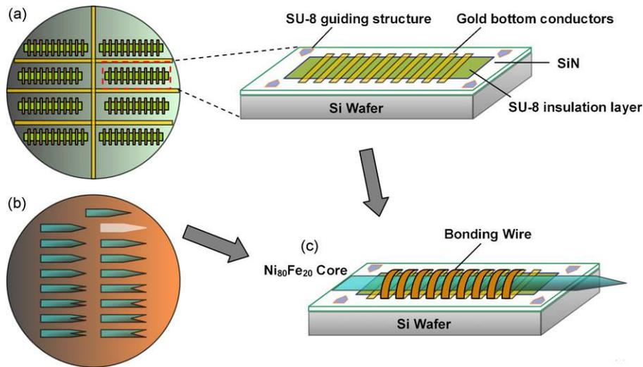
Fig. 3. An illustration of the fabrication process of the micro electromagnetic probe: (a) fabrication of gold bottom conductors and SU-8 insulation and guiding structures; (b) fabrication of the Permalloy magnetic cores; (c) assembly of the magnetic core on the chip and placement of the top conductors with wire bonding.
