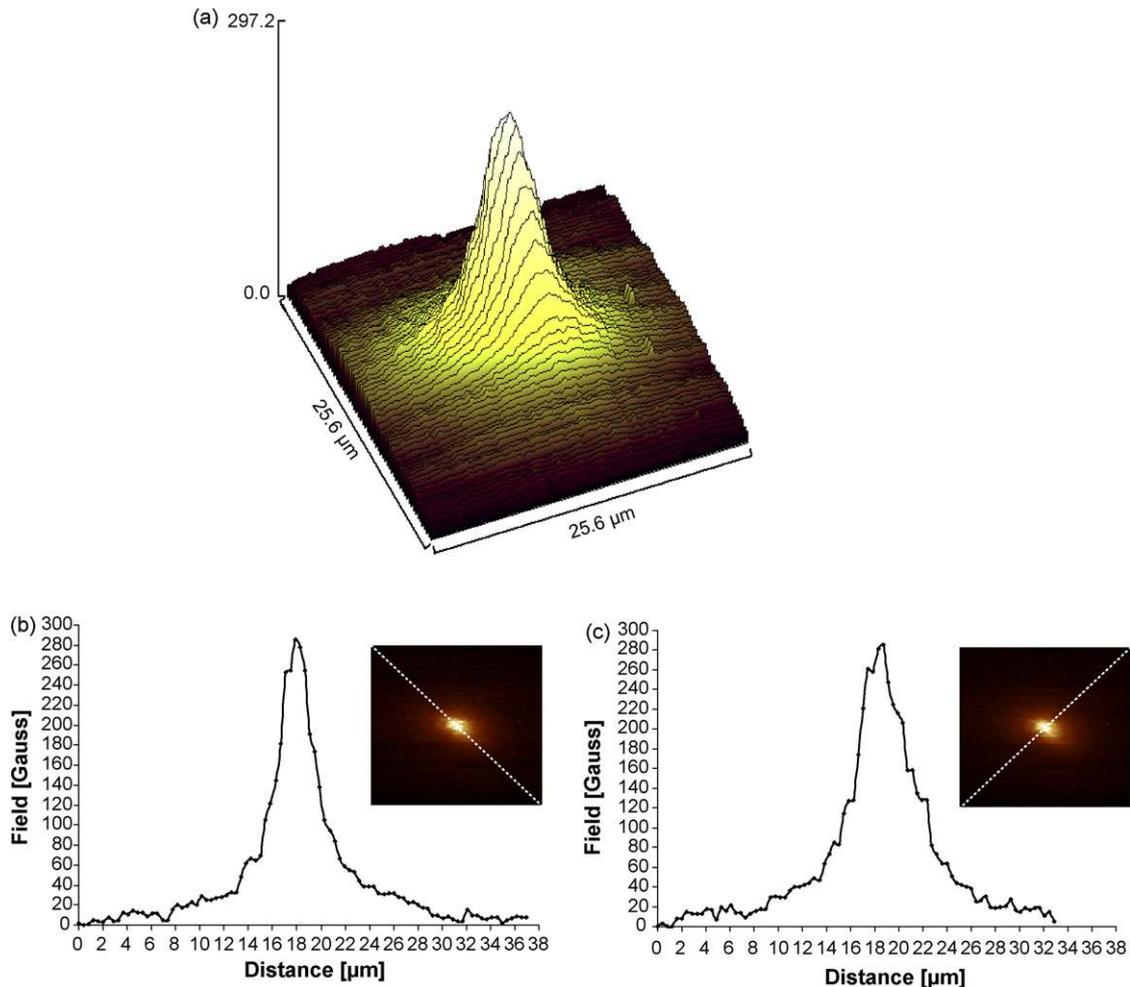
Fig. 9. Measured spatial distribution of the magnetic field output (the component parallel to the axis of the probe) with an input current of 300 mA: (a) surface plot; (b) and (c) axial field plots along the diagonals of the probe tip obtained from the cross-sectional field distribution.
