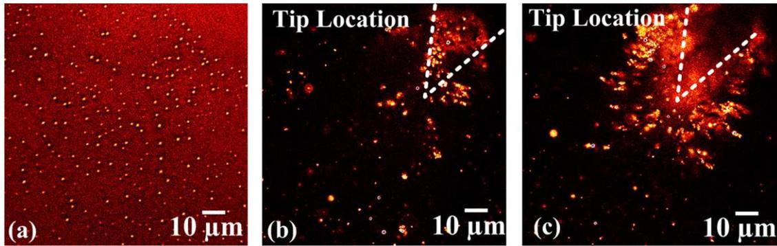
Fig. 10. Manipulation of fluorescent magnetic particles using the developed electromagnetic probe (observed under a fluorescence microscope): (a) Magnetic particles stay in their equilibrium position; (b) and (c) After the probe is turned on, magnetic particles move steadily towards the probe tip.
