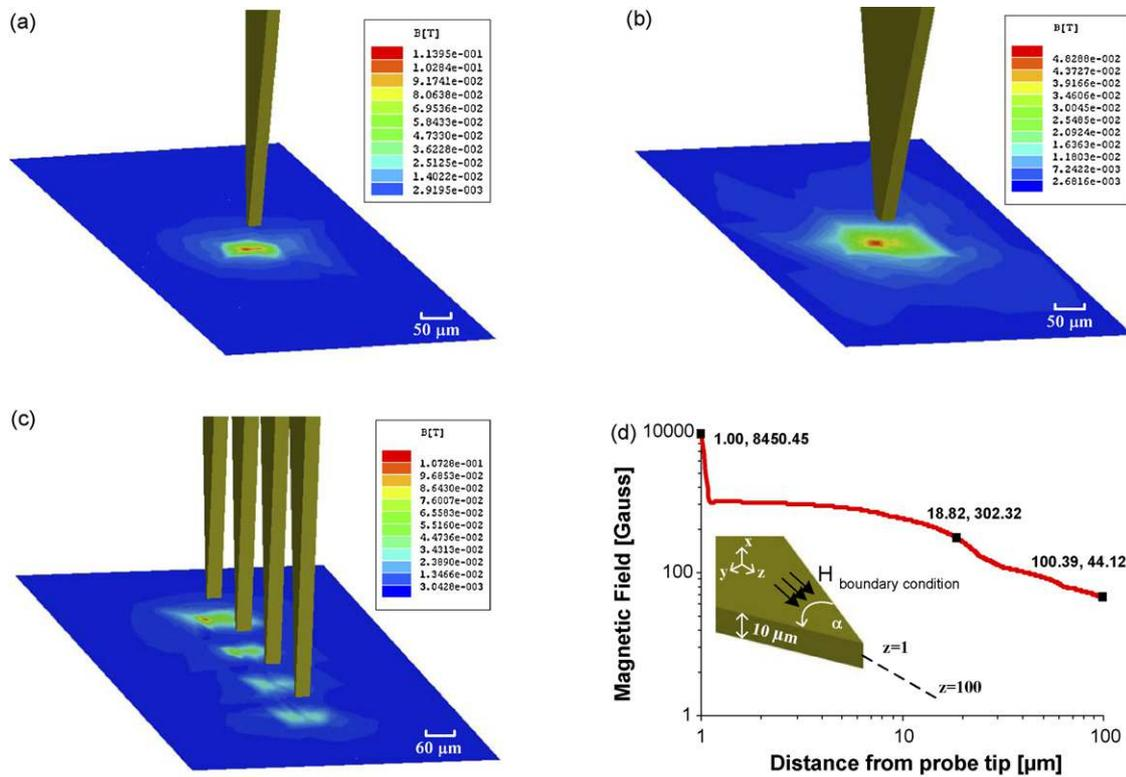
Fig. 2. Simulated magnetic field distribution of different probe tip designs: (a) Field distribution of a probe tip with a taper angle of 15.2°; (b) field distribution of a probe tip with a taper angle of 43.6°; (c) field distribution of a four-tip design; (d) Line plot in log–log scale showing the rapid fall of the magnetic field with respect to distance from the probe tip for a probe design with taper angle 15.2°, shown in the inset is a pictorial representation of the simulation conditions.
