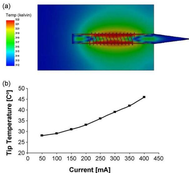
Fig. 6. (a) Finite element simulation showing the temperature distribution on the micro electromagnetic probe under 300 mA input current; (b) plot of the probe tip temperature under different input current levels.
