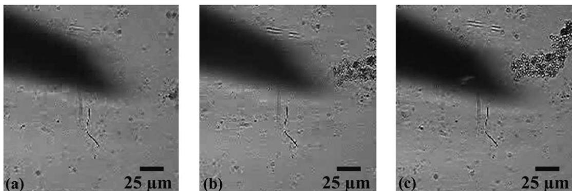
Fig. 11. Manipulation of magnetic particle agglomerate: (a) At  $t=0$  s, magnetic field is applied; (b) At  $t=2$  s, magnetic agglomerate moves toward the probe tip; (c) At  $t=4$  s, magnetic agglomerate is captured.
