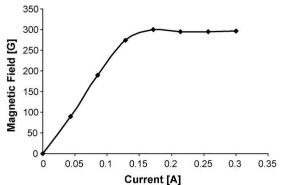
Fig. 7. Magnetic field output  $20 \mu\text{m}$  from the tip of the tested micro electromagnetic probe as a function of input current.
