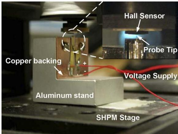
Fig. 5. Scanning Hall probe microscope setup for micro electromagnetic probe characterization. The gap between the probe tip and Hall sensor is estimated to be  $\sim 20 \mu\text{m}$ .
