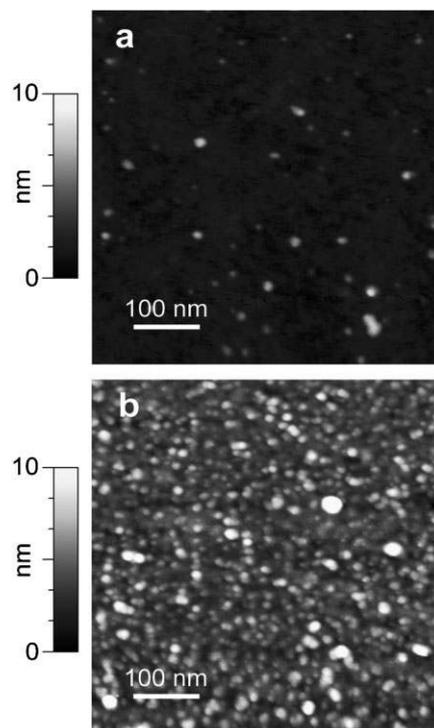
**Figure 4.** AFM images taken on the a) irradiated and b) nonirradiated area, demonstrating how particles graft solely onto the nonirradiated areas.
