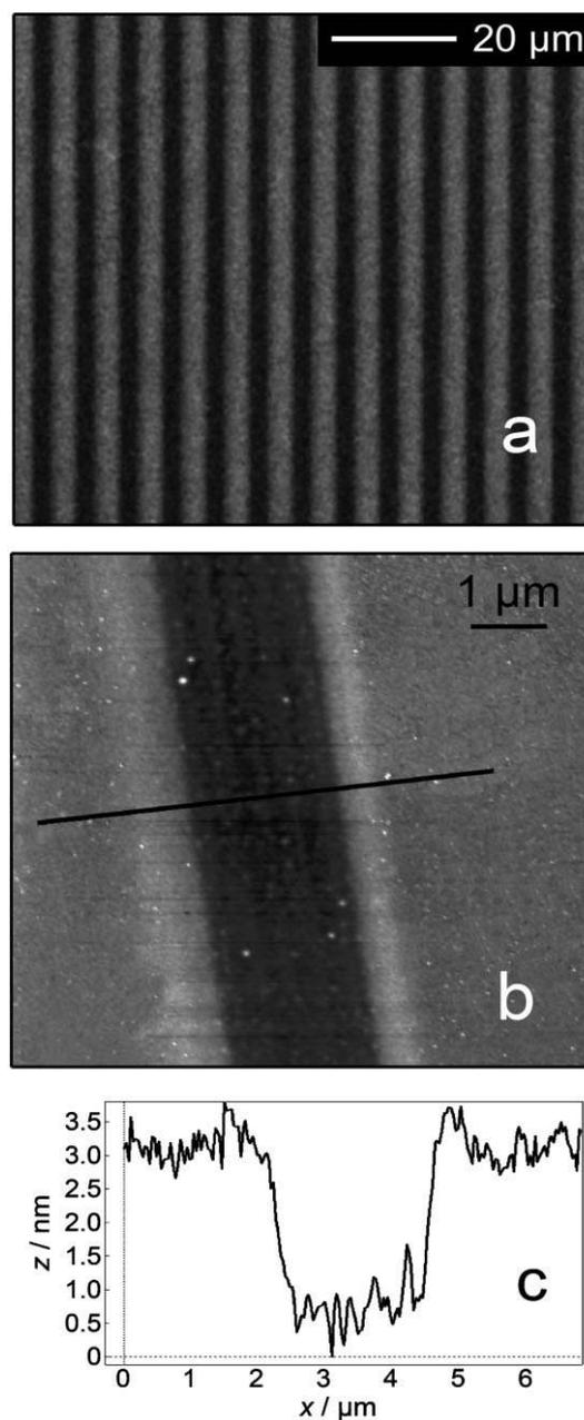
**Figure 2.** a) SEM micrograph showing the patterning of the surface before the deposition of the nanoparticles: light gray stripes are nonirradiated whilst the darker ones were irradiated by the ion-beam. b) AFM image focalized on one irradiated stripe. c) AFM profile taken along the reference line in (b): the 3 nm step shows the groove in the organic layer made by FIB.
