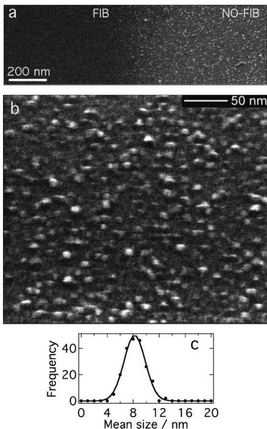
**Figure 3.** SEM imaging of the patterned monolayer. a) Micrograph demonstrating how particles graft solely onto the nonirradiated areas. b) High-resolution SEM image of (CsNiCr)-PBA nanoparticles deposited on unpatterned area. c) Gaussian distribution of the sizes of the particles with mean value  $l^* = 8.0 \pm 2.0$  nm and standard deviation  $\delta = 4.6$  nm.
