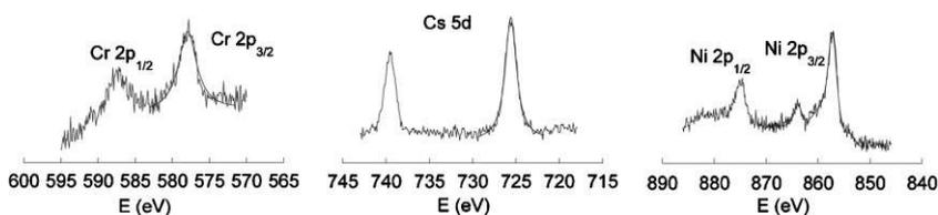
**Figure 6.** XPS spectra of the monolayer of (CsNiCr)-PBA nanoparticles taken at the Cr, Cs, and Ni edges.
