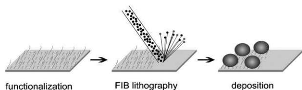
**Figure 1.** Schematic drawing showing the fabrication procedure. Upon the functionalization of the Si(100) surface, portions of ligand are removed by the FIB patterning. The sample is then rinsed with methanol to wash off the debris of the sputtering process. In the last step, the deposition is carried out by submerging the sample in the solution of (CsNiCr)–PBA nanoparticles.
