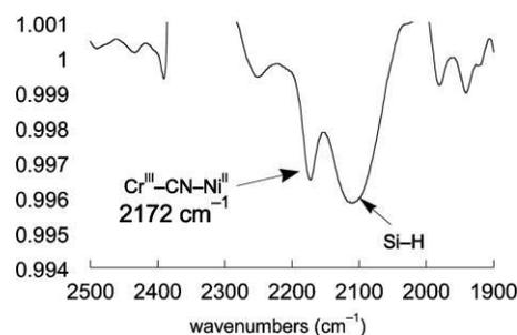
**Figure 5.** ATR FTIR spectrum of a monolayer of the (CsNiCr)-PBA nanoparticles on functionalized Si(100).
