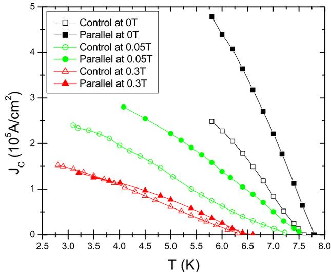
FIG. 5. (Color online) Average critical current density  $J_C$  for current parallel to the stripes and for the control sample for ( $\mu_0 H = 0, 0.05, 0.3$  T).
