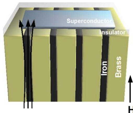
FIG. 1. (Color online) Schematic design of the magnet-superconductor hybrid system and sketch of the magnetic field distribution.
