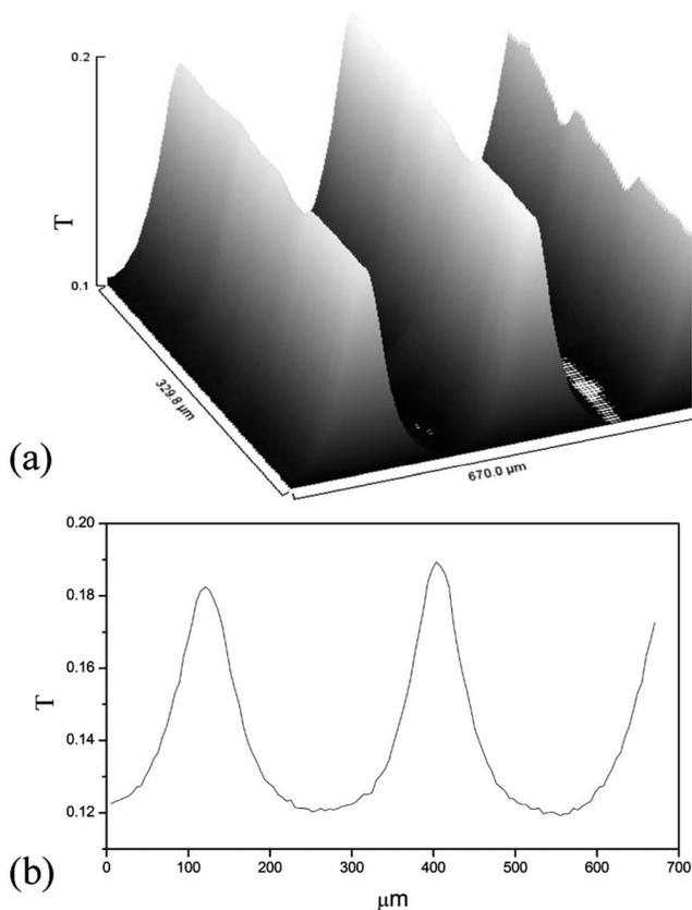
FIG. 2. (a) Normal component of magnetic field about  $10 \mu\text{m}$  above Fe-brass laminate measured with SHPM. (b) SHPM line scan perpendicular to the magnetic field stripes in (a).
