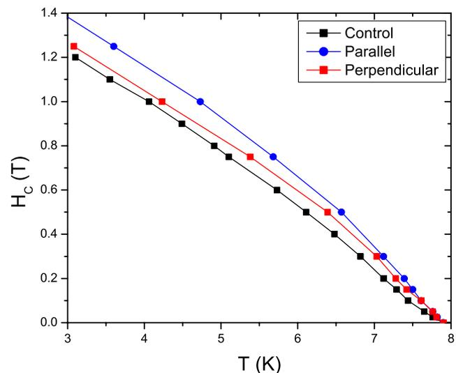
FIG. 4. (Color online)  $\mu_0 H_{C2}(T)$  for the current parallel and perpendicular to the stripes and for the control film.
