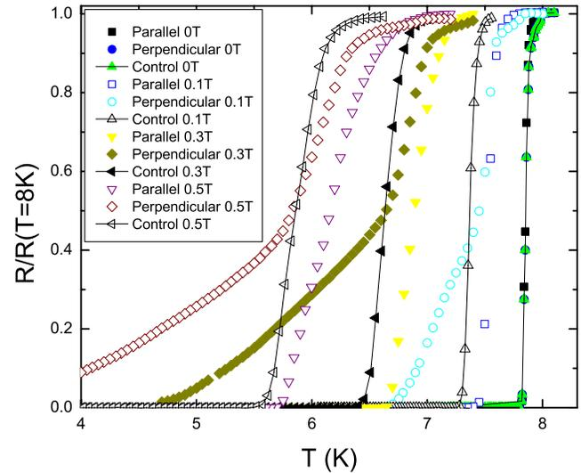
FIG. 3. (Color online) Normalized resistance curves  $R(T)/R(8 \text{ K})$  for the current parallel and perpendicular to the magnetic stripes and for the control sample for  $\mu_0 H=0, 0.1, 0.3,$  and  $0.5 \text{ T}$ .
